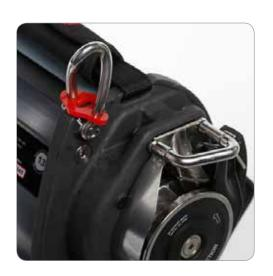
1) Connect the twisted shackle with the rubber fixation, as shown, to the secondary connection point of the ascender.
