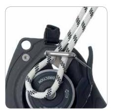
Form a loop on the rope and push it through the rope guide just above the rope grab.
