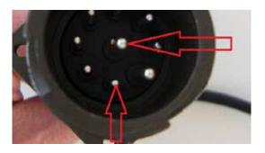
2) Measure the voltage (on pins A and I as shown in the picture) of the charger at the battery connector with a common voltmeter, when the charger is connected to the wall socket. It shall be 39,6 V if the charger is ok.
