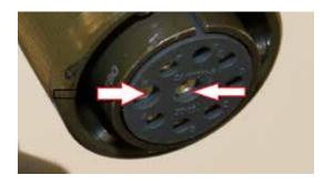
1) Measure the voltage (on pins I and H as shown in the picture) of the battery with a common voltmeter. It shall be 37,2 V when the battery is fully charged.
